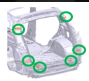
Bamboo joint structural reinforcement
